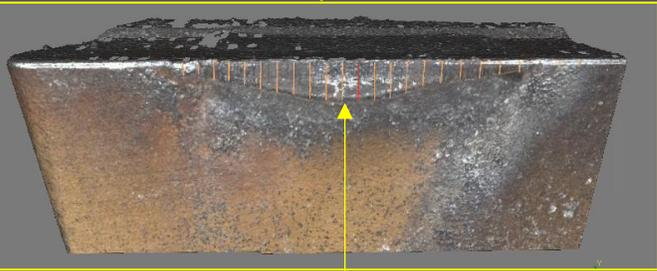
Tool wear on the relief side of insert
