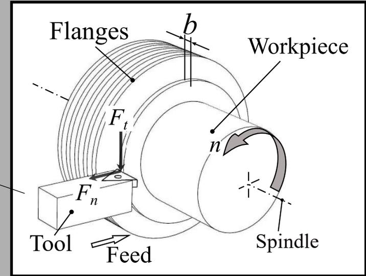
2D Orthogonal Cutting Operation
