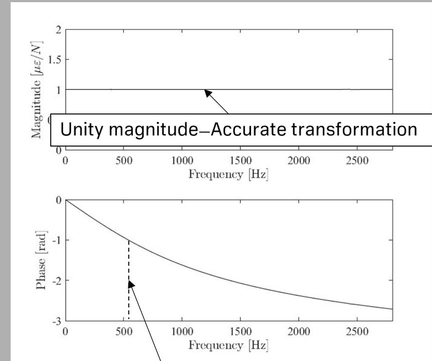
Approx. linear phase until 650Hz, low-pass filter with a cutoff at 650Hz is applied to the inverse-filtered signals.
