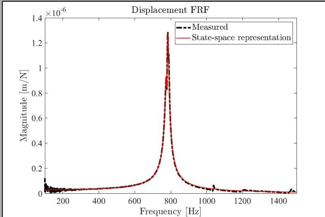
Using measured FRF to fit **State-space model** by MATLAB's System Identification Toolbox
