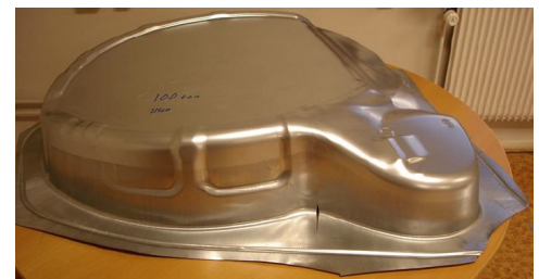
Volvo Cars component displaying fracture due to non-linear strain paths.
