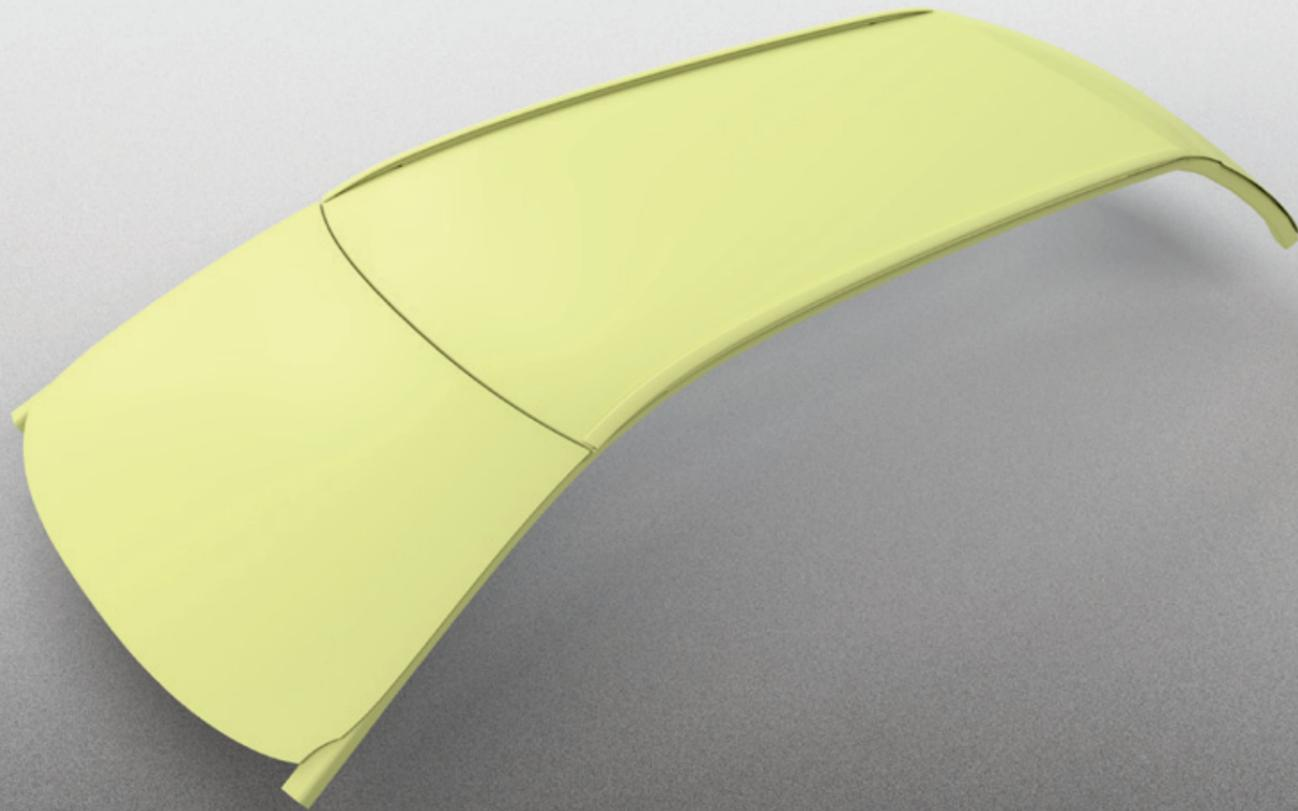
The concept of modularization was the focal point of the roof team's design process. Not only does it enable more efficient production, it also creates the opportunity for integration of parts such as sun cells, ventilation fans, electronics and other interior parts. Furthermore, it reduces the number of fasteners on the vehicle body and allows for a more efficient way of manufacturing the rest of the car structure due to better access and favourable geometry.
