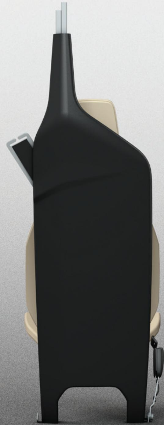
The innovative solution proposed for this was a seat fixed to a vertical structure that would adapt to each driver's height and weight. The vertical structure is attached to larger-lightweight frame that gives support to the entire car structure. The frame distributes the weight via multiple connection points to the body structure thereby enabling a lightweight seat framework.
